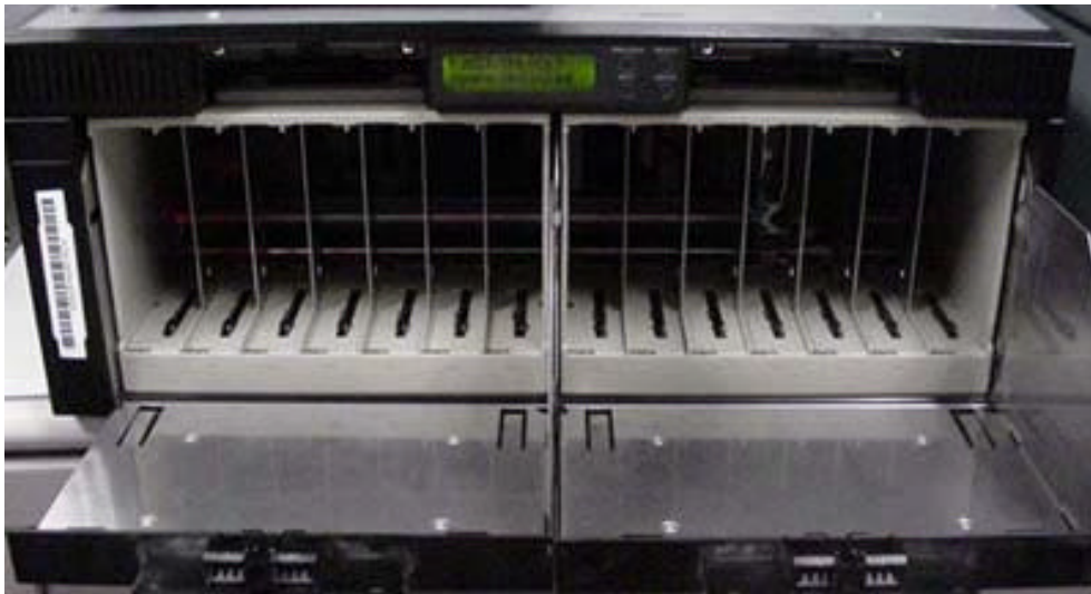
Figure 4: The 3502-R14 with both magazines installed. Behind the magazines are the autoloader arm and the tape drives.
