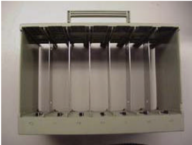
Figure 1: The 3502-x14 Magazine with no populated slot and no metal tabs engaged.
