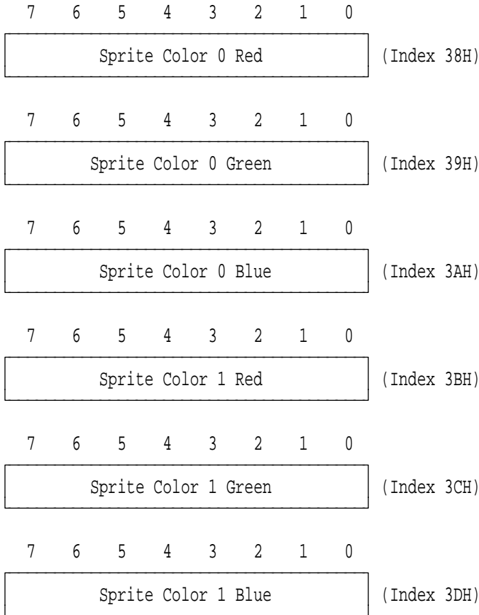
Figure 3-67. Sprite Color Registers, Indexes Hex 38– 3D
