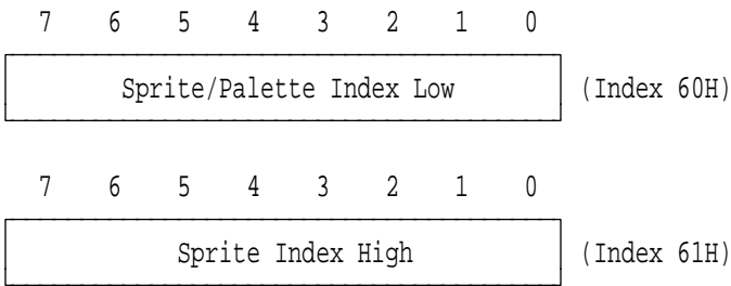
Figure 3-86. Sprite/Palette Index Registers, Indexes Hex 60 and 61
