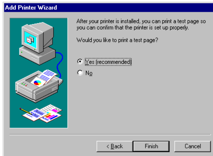
Figure 7-10. Add Printer Wizard Dialog Box - Printing a Test Page
