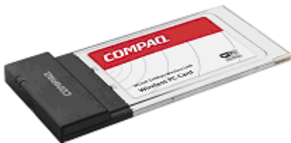
Figure 4: Compaq WL110 wireless LAN (802.11b)
