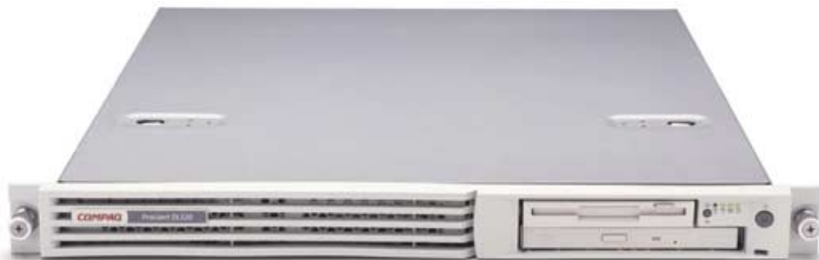
Figure 1: Compaq ProLiant DL320 ultra-dense server
