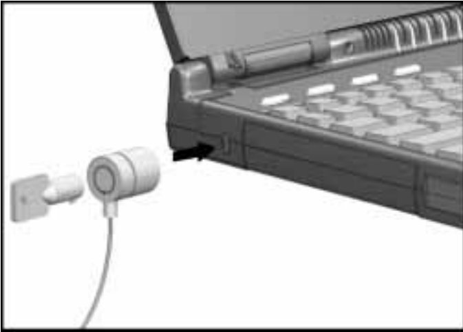
Installing a Cable Lock
