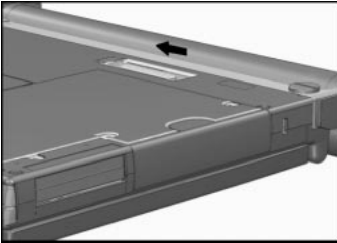
Opening the Expansion Slot Cover
