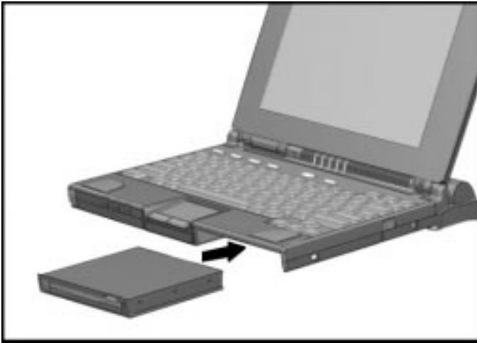
Inserting the Diskette Drive into the DualBay
