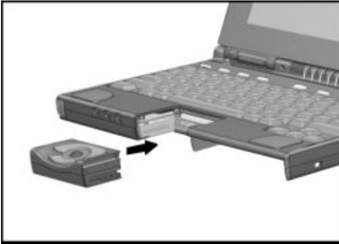
Installing the Pointing Device (Trackball)
