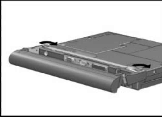
Turning Thumbscrews to Tighten Handle
