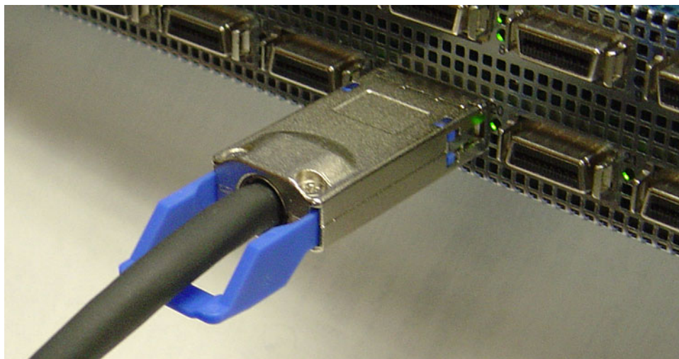
Figure 2-13: Fully Installed IB Cable with Pull Connector
