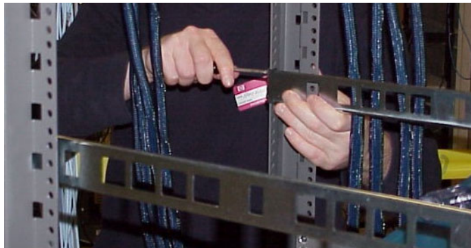
Figure 2-5: Secure Rail Bracket to Rack with Screws
