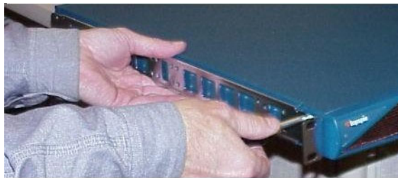
Figure 2-3: Attaching One Rail to Switch Chassis
