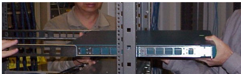
Figure 2-6: Sliding the Switch Into the Rack
