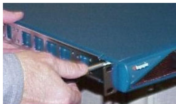
Figure 2-9: Fasten Bracket to Switch Chassis
