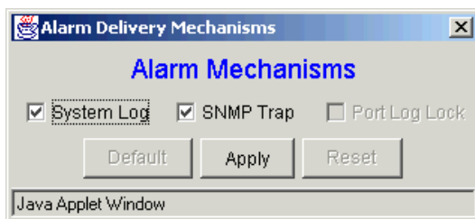
Figure 2-1: Alarm Mechanisms dialog box
