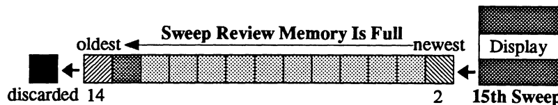
Figure 5 - The 15th sweep was triggered. This forced the memory to discard the first sweep (black box) to make room for the 14th sweep.
