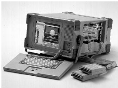
Figure 1: HP E4829B integrated into the BSTS system
