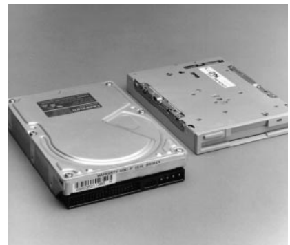
Figure 23. Both the HP 16500C and 16505A come with a built-in hard disk drive and a 1.44-MB floppy disk drive.
