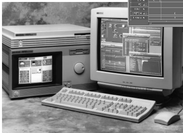
Figure 4. The HP 16505A prototype analyzer is a measurement server that uses the HP 16500C's real-time measurement power. It adds a large-screen, windowed display and powerful analysis tools.
