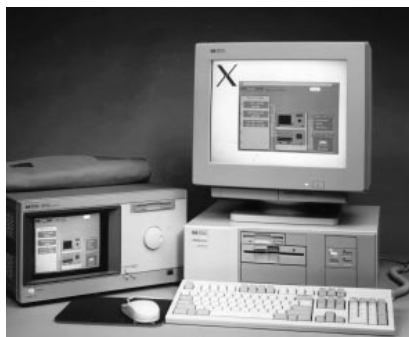
Figure 20. Control the HP 16500C remotely using the X-windows interface.
