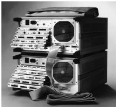
Figure 17. Add more HP 16500-series measurement modules to your HP 16500 logic analysis system with the HP 16501A expansion frame.
