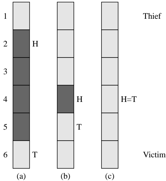
Figure 2-7: The three cases of the ready deque in the simplified THE protocol. A dark entry indicates the presence of a frame at a certain position in the deque. The head and the tail are marked by T and H.
