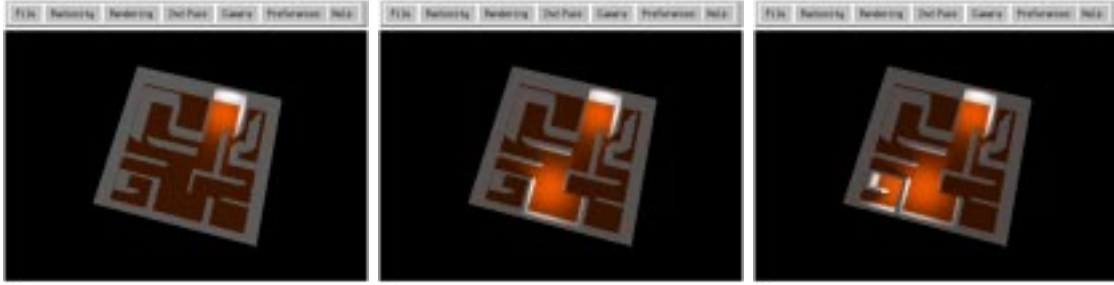
Figure 10-2: The first three iterations of the rad program on a maze scene. At each iteration, the program refines its formfactor estimates for the patch where the error is greatest. In the first few iterations, the error is greatest near the light sources, so the program appears to be “lighting up” the lights one by one.
