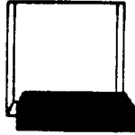
Figure 6.9: The black polyhedron contains sensed positions that terminate the motion of Figure 6.8 in the interior of the cube bottom.
