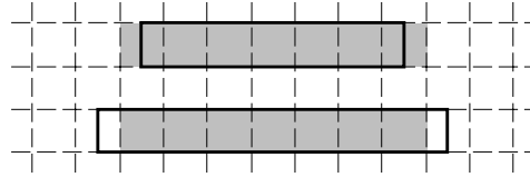
Figure 5-6: The effect of quantization errors on the length of a row of pixels.
