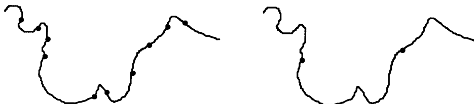
Figure 20. Smoothing the curvature removes small zero crossings, and preserves only the larger scale inflection points.
