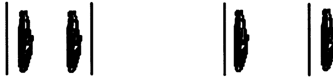
Figure 27. Spatial configurations of edge segments with similar intensities on one side, a) likely to be part of the same object, b) unlikely to be part of the same object.
