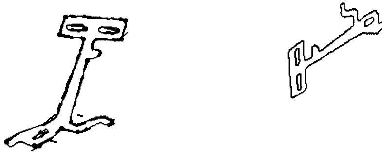
Figure 53. Match of a model to a bent instance using the adjacent parts method.
