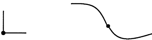
Figure 34. Class II features define a point and an orientation. A pair of matching features is sufficient for alignment.
