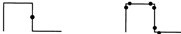
Figure 19. Segmenting a contour, a) at inflections only, b) at ends of straight segments and inflections.
