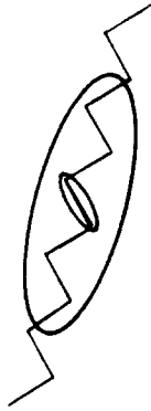
Figure 18. At a given spatial location, the jagged contour can give rise to edge primitives with different orientations at different scales.
