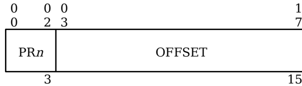
Figure 6-7. Format of Instruction Word ADDRESS When Bit 29 = 1
