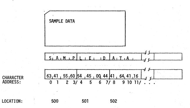
The second part of the illustration shows the relative position of each character in the buffer. The high-order bit of each character position in a word is occupied by the high order bit of the character residing there. This can be seen by part three (3) which gives the octal value of each buffer location after the card code has been converted to trimmed ASCII.
