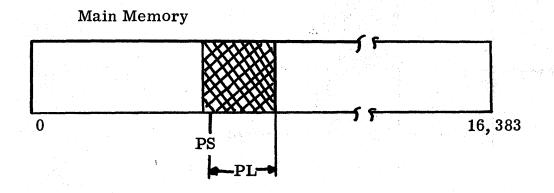
The area of main memory that the file is segmented into is defined by PS and PL. PS is the main memory address of the buffer area and PL is the number of sectors available for this buffer. PS and PL must be assigned values by the user; PMFH entries in words 2-5 are initialized and maintained by the file procedures.
