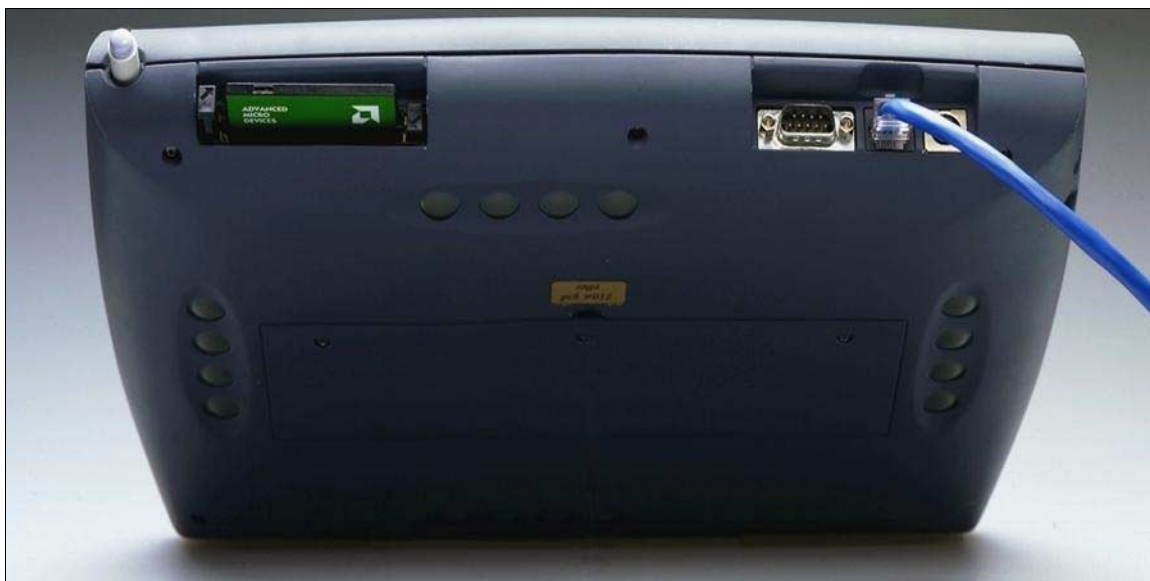
Figure 4: View showing the pen in its holder, a Flash card in a slot and the Ethernet/power tether
