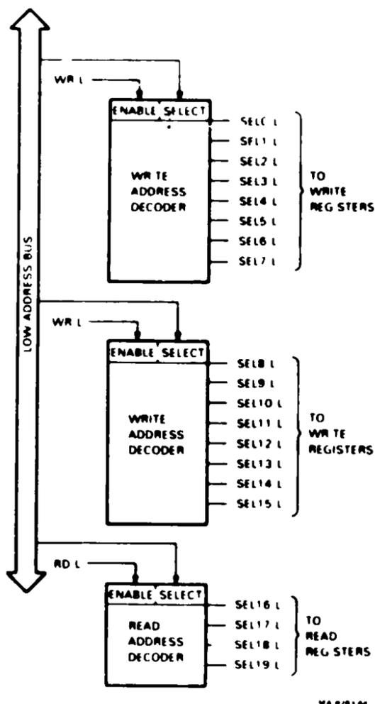
Figure 2-9 Address Decoders with Low Address Bus
