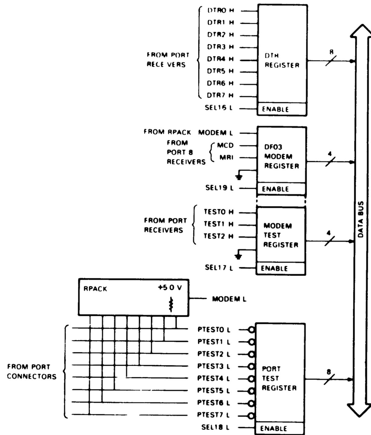
Figure 2-14 Read Control Registers with Data Bus
