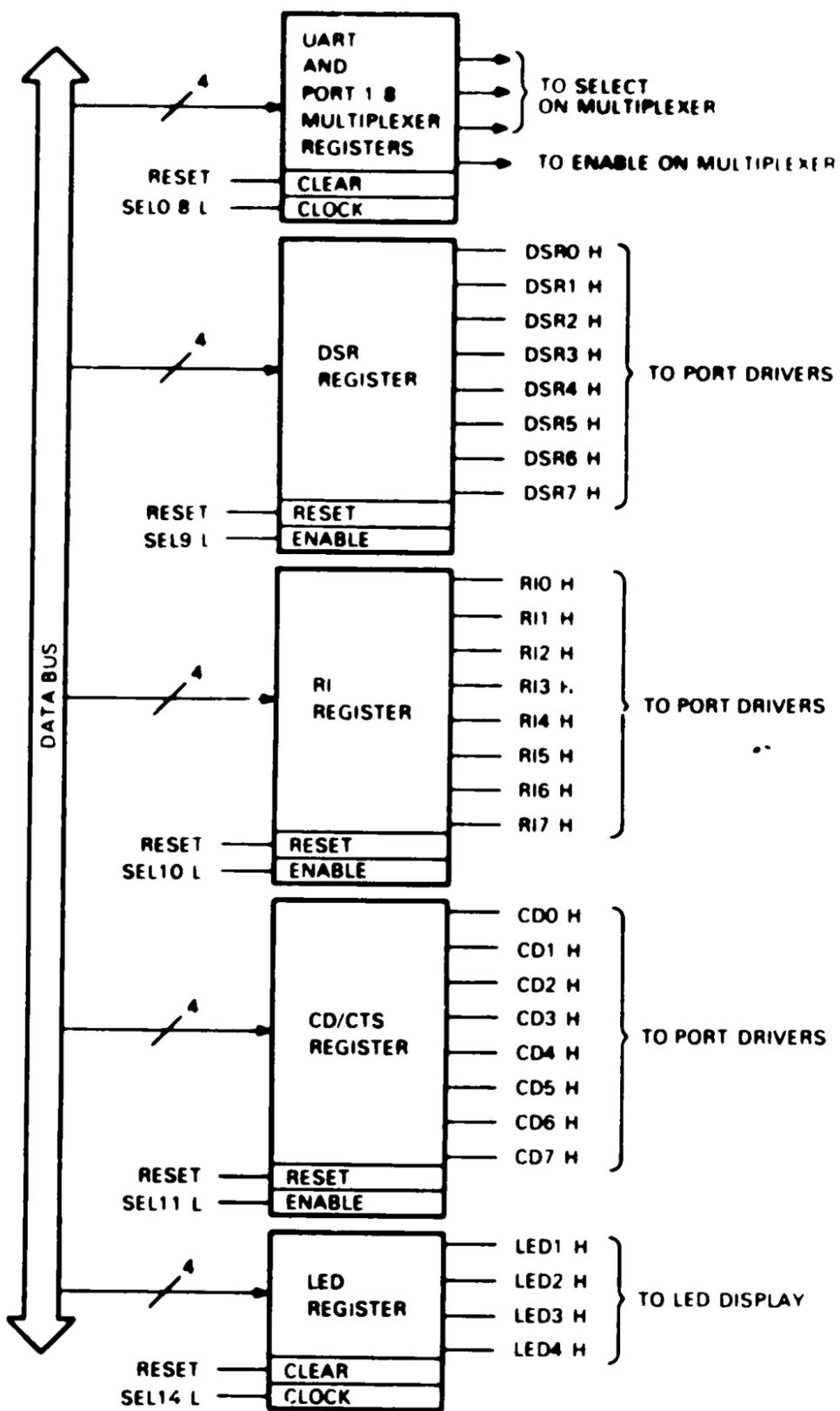
Figure 2-13 Write Control Registers with Data Bus
