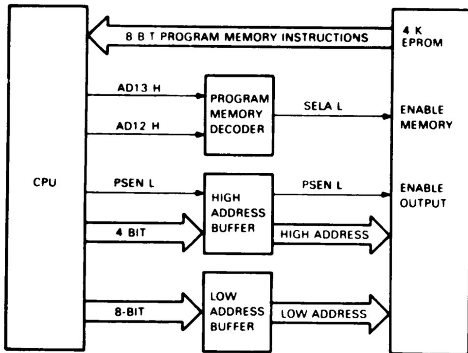
Figure 2-6 EPROM Block Diagram
