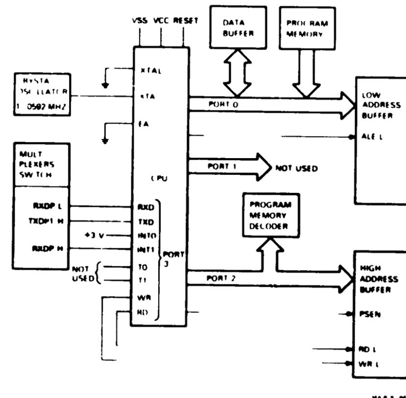
Figure 2-3 CPU Block Diagram
