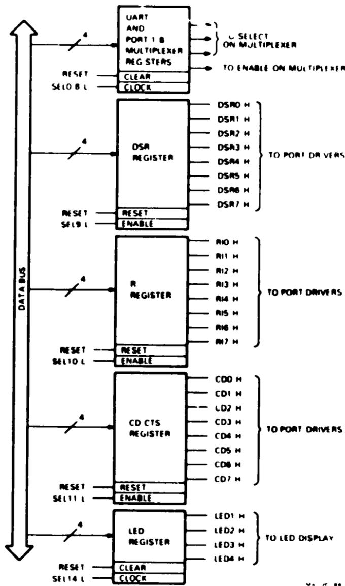
Figure 2-13 Write Control Registers with Data Bus
