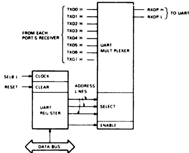
Figure 2-11 UART Multiplexer with Control Register
