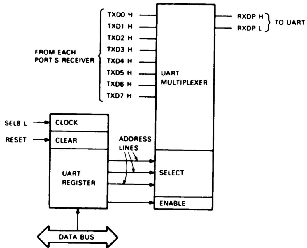
Figure 2-11 UART Multiplexer with Control Register
