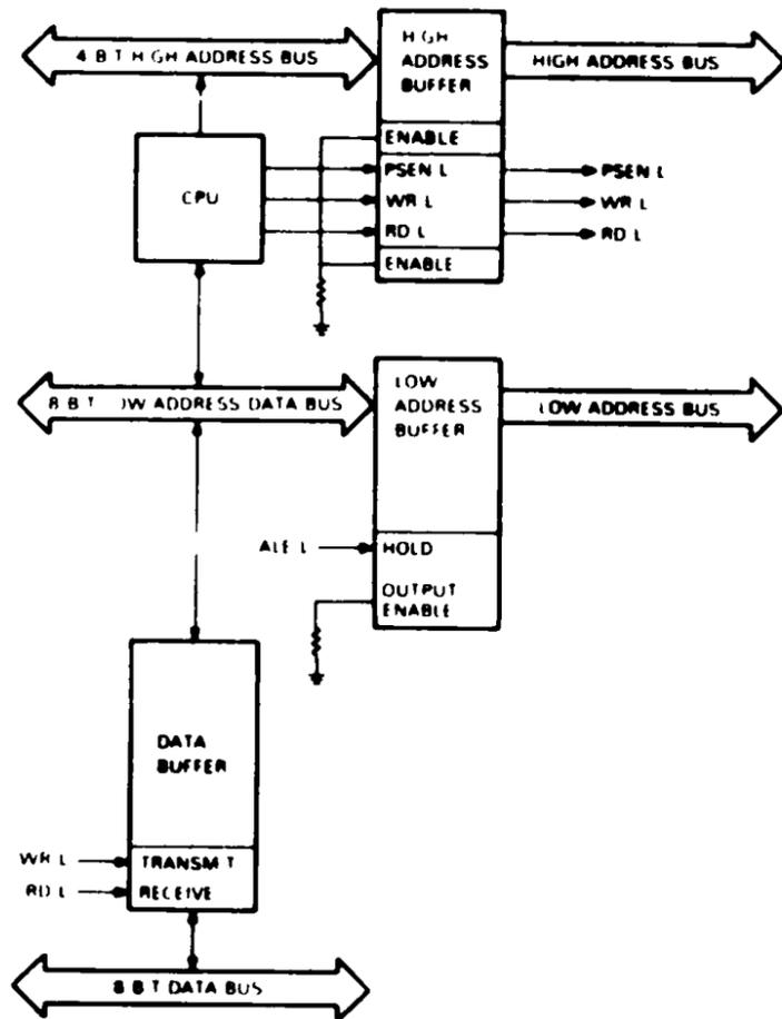
Figure 2-8 System Block Diagram with Buses and Buffers
