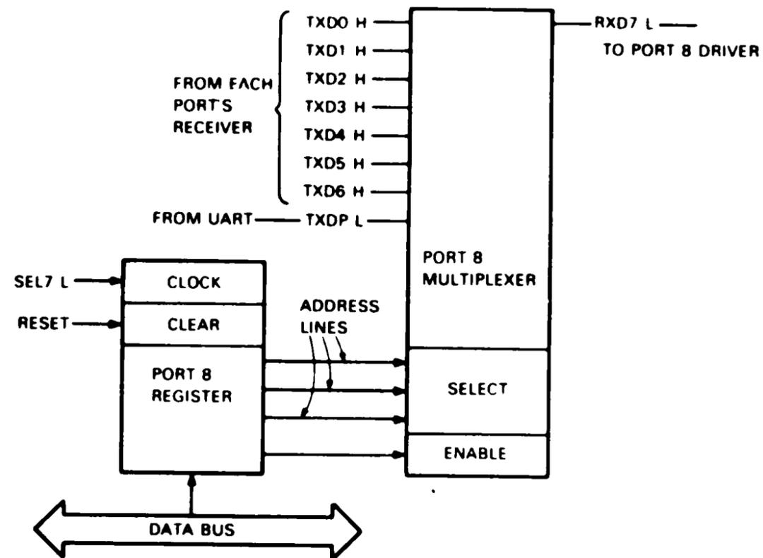
Figure 2-12 Port 8 Multiplexer with Control Register
