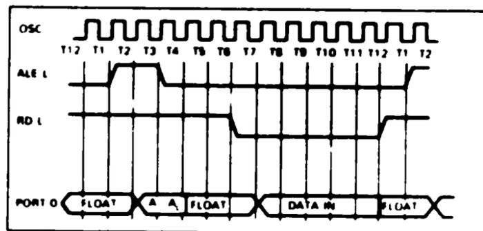
Figure 2-15 Data Read Cycle Timing
