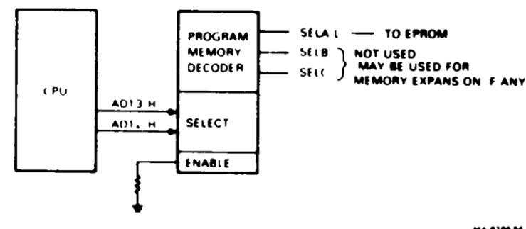
Figure 2-10 Program Memory Decoder Block Diagram
