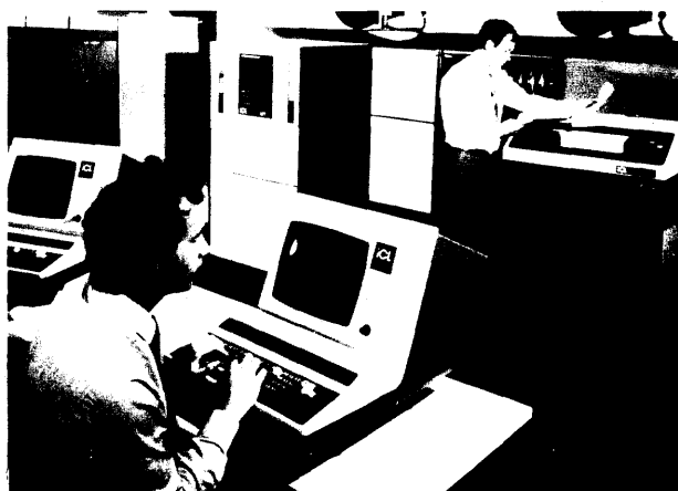
The ICL 2966 mainframe computers can be configured with single or dual processors having up to 32M bytes of store, each.
