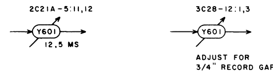
Figure 10. Adjustable Capacitive Delays
