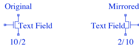
Figure 5-12 Mirrored Transistor, Note Reversal of Two Attributes
