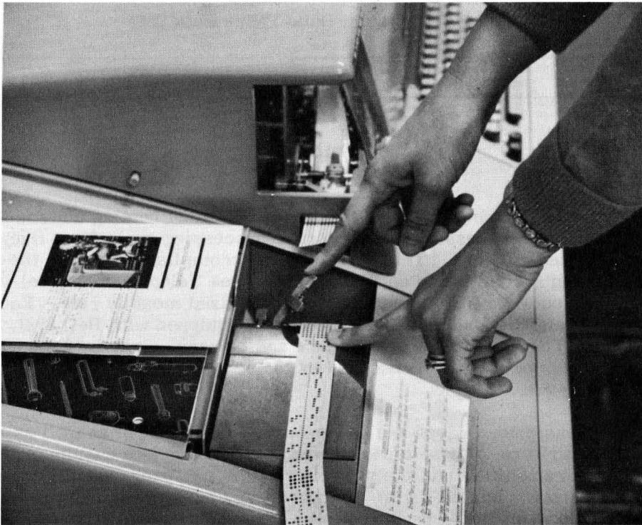
Fig. 1 - MODEL 35 TELETYPEWRITERS produce punched paper tapes which, when transmitted, between Wiegand headquarters and outlying warehouses, provide computer and Flexowriter input for the company's speedy order processing system.
