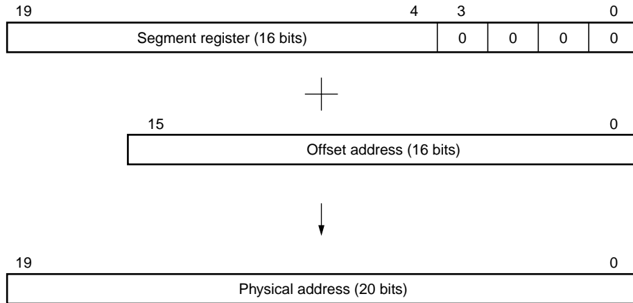
Figure 3-7. Relationship between Segment Register, Offset Address and Physical Address
