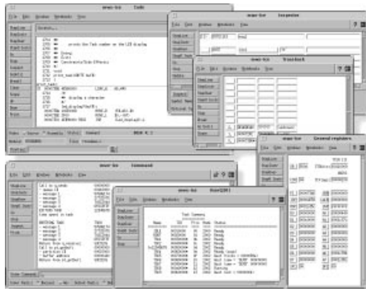
The multi-windowed debugger speeds development with simultaneous display including (clockwise from upper left): symbolic representation of structure elements; stack values; call tracing; register values; interleaved source and assembly; and pure source code.
